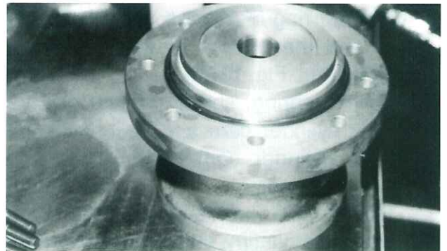
Fig. 131 Assembling Unloader Piston (High-stage)
